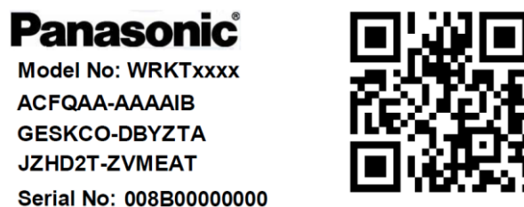
Figure 1 KNX Secure Device Certificate Label
